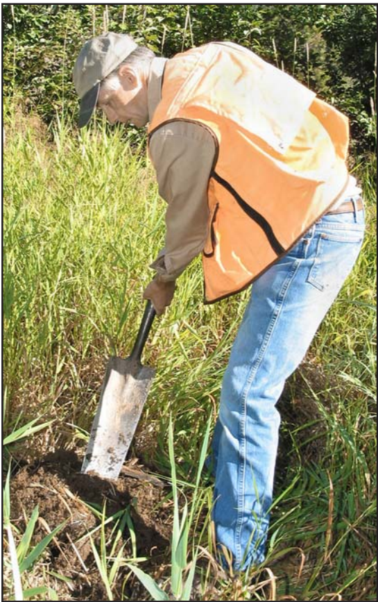
Rayner, digs a hole about 18 inches deep to get a soil sample that will help him determine the wetland delineation (boundary) of a location along the Spokane River just east of Coeur d'Alene.
