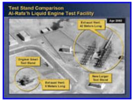
As part of this effort, another little piece of evidence, Iraq has built an engine test stand that is larger than anything it has ever had. Notice the dramatic difference in size between the test stand on the left, the old one, and the new one on the right. Note the large exhaust vent. This is where the flame from the engine comes out. The exhaust vent on the right test stand is five times longer than the one on the left. The one of the left is used for short-range missiles.
