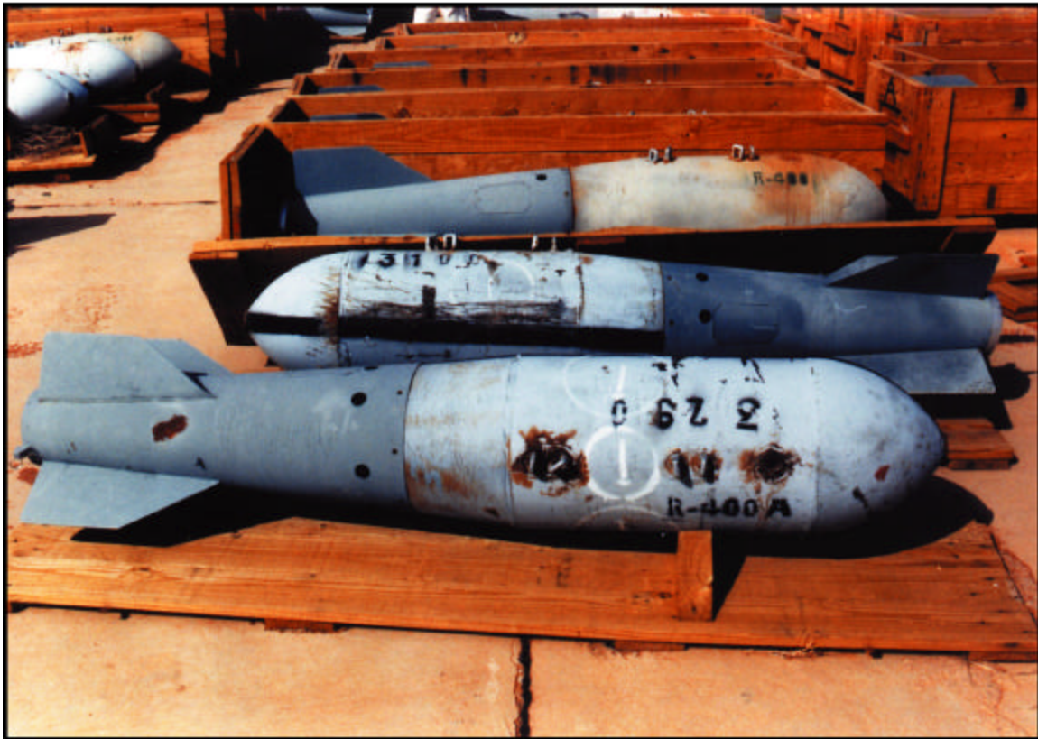
Two R-400A bombs in foreground photographed by UNSCOM inspectors at Murasana Airfield near the Al Walid Airbase in late 1991 bear markings indicating they were to be filled with botulinum toxin. Other bombs appear to have markings consistent with binary chemical agent fill. This evidence contradicted Iraq's declarations that it did not deploy BW munitions to operational airbases and that it destroyed all BW bombs in July 1991—declarations that were subsequently retracted in the face of overwhelming evidence to the contrary.
