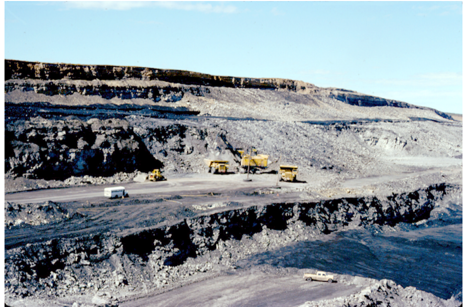
Figure 11. Colowyo coal mine in the northern part of the Danforth Hills coal field. The mine produces coal from FGF and FGG zones (as many as nine beds) in the Fairfield coal group by dragline and truck-and-shovel methods.
