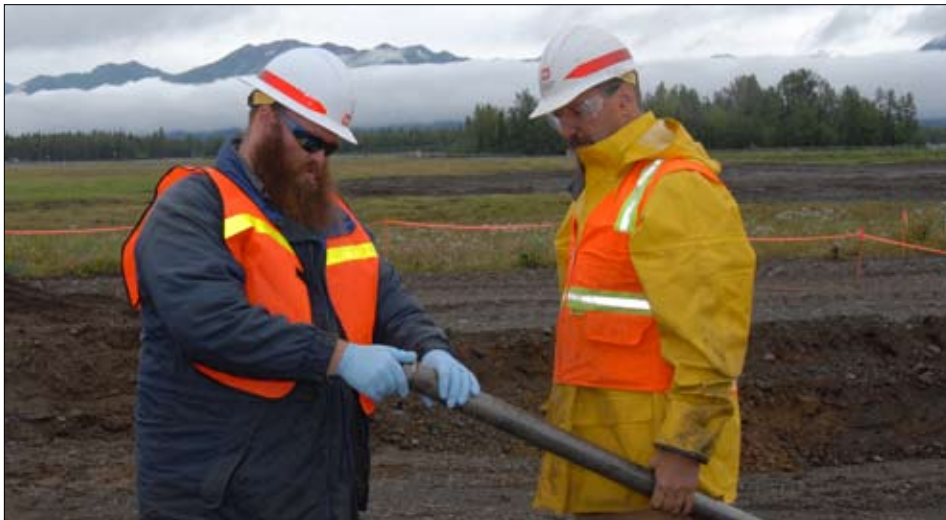
Sean Benjamin (left), a chemist in the Materials Section, pulls a plastic sleeve from a sample tube held by Bob Glascott, an environmental scientist in the Environmental and Special Programs Branch, during a soil sample investigation at Elmendorf Air Force Base to identify potential pesticides on a construction site.
