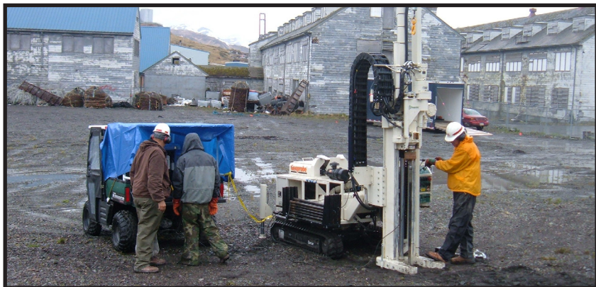
Alaska District uses laser-induced fluorescence at the Amaknak Formerly Used Defense Site at Dutch Harbor.
