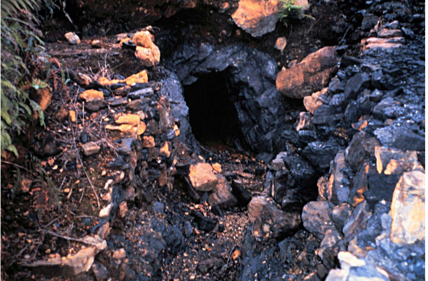
Figure 6. View of a typical coal mine in Guizhou Province, China. Mine opening is approximately 0.5 m wide. Note the absence of timber supports. Coal in the vicinity of this mine contains 35,000 parts per million (ppm) arsenic (As)! U.S. coal has, on average, 20 ppm As. Also nearby is a small gold mining operation. Some of the coal samples have ore grade concentrations of gold (600 ppb to 3 ppm in the coal ash).
