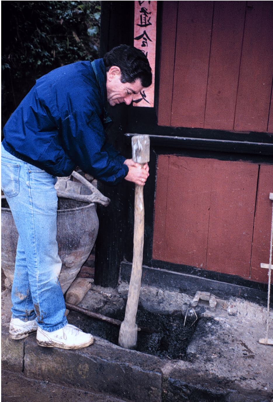
Figure 18. Villagers prepare briquettes by pulverizing moist coal containing 100 - 200 ppm F (in contrast, most coals worldwide have 50 - 100 ppm F). The pulverized coal is then mixed with clay to form briquettes to control combustion temperature and timing. The clay used is the residue of intense weathering of the local limestone. These local residual clays are typically enriched in F (commonly > 1,000 ppm).
