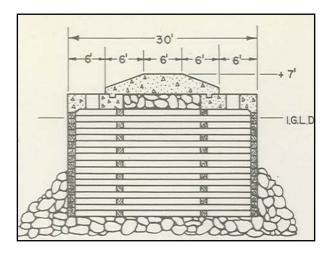
Several types of breakwaters have been constructed in the Great Lakes. The oldest and largest group used timber crib core sections. Timber cribs are wooden frames that were constructed on shore, floated into position, and filled with rocks to sink them into place. Most timber cribs had a concrete or stone superstructure added later, and some have added steel sheetpile reinforcement.
