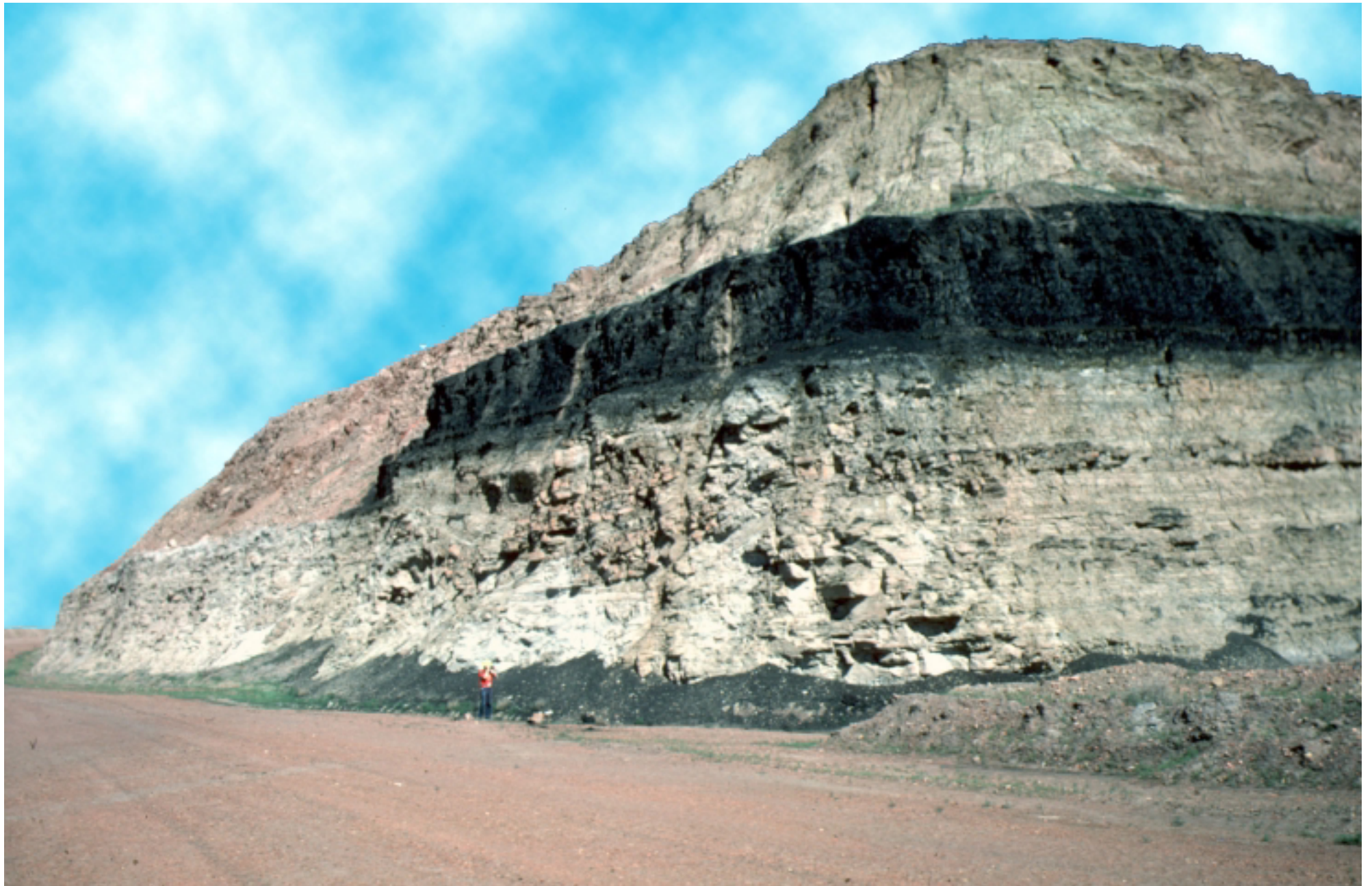
Figure PS-21. Clinker (orange-red at the left of the picture) of the Anderson or Dietz 1 coal bed (at the right of the picture ) on the Decker coal mine in Montana. Burning has reduced the reserve of the Anderson coal bed. Photograph by R.M. Flores.
