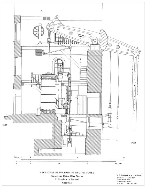
A CAD-generated drawing of the Cornish beam engine brought to Goonvean in 1910 to pump Goonvean Clay Works in Cornwall, England. Surveyed using a reflectorless, Total Station EDM theodolite, the information captured electronically and by hand measurement in such an exercise can be manipulated and printed in 2D, at any scale and showing arrangement or detail as required. Drawing by N.R. Fradgley and M.J. Williams for English Heritage, 1999.
