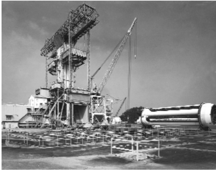
The static test tower in the East Test Area, Marshall Space Flight Center. The first stage of a Saturn I booster is on its side to the right of the static test tower. Photo by Jet Lowe, 1996.
