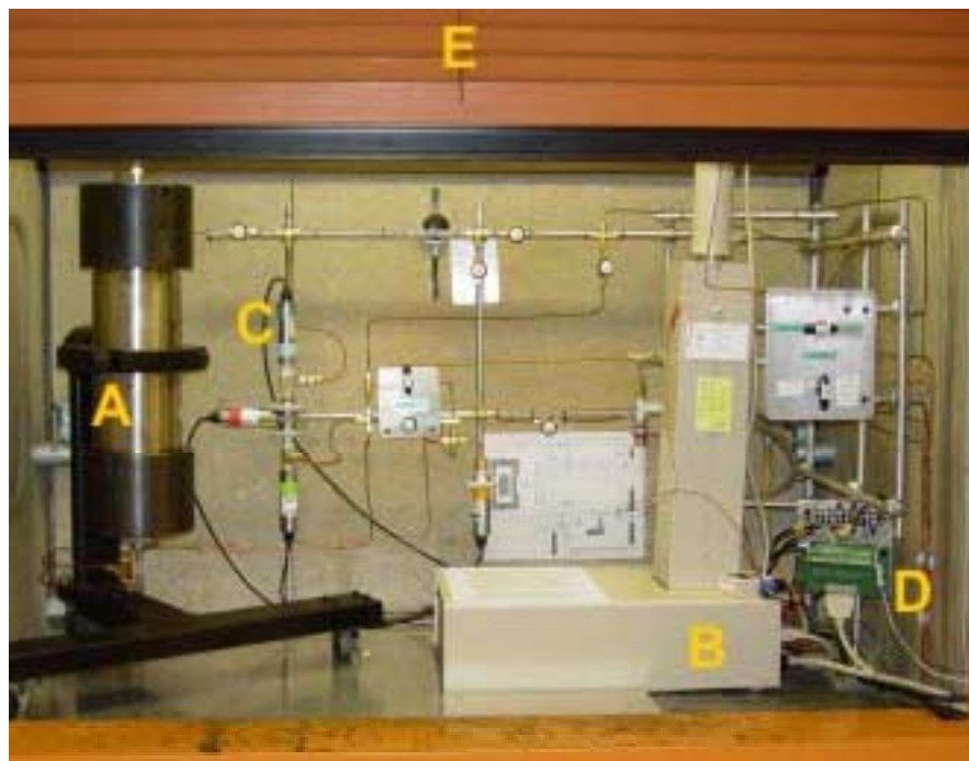
Figure 1. — View of the instrumentation. A is the reactor in which coal core samples will be placed; B is the injection pump for metering gas to the reactor; C are several pressure transducers; D is part of the data acquisition board to which instrumentation is connected, and E is the fume hood in which the apparatus is located, allowing safe venting of gases.
