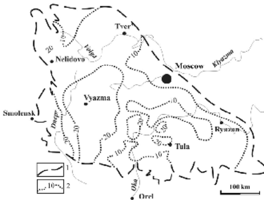
Figure 1. — Bobrikovsky horizon thickness in the Moscow lignite basin (adopted from M.K. Makhlina, and others, 1993). 1) the Moscow lignite basin regional boundaries; 2) Bobrikovsky horizon isopach, m.
