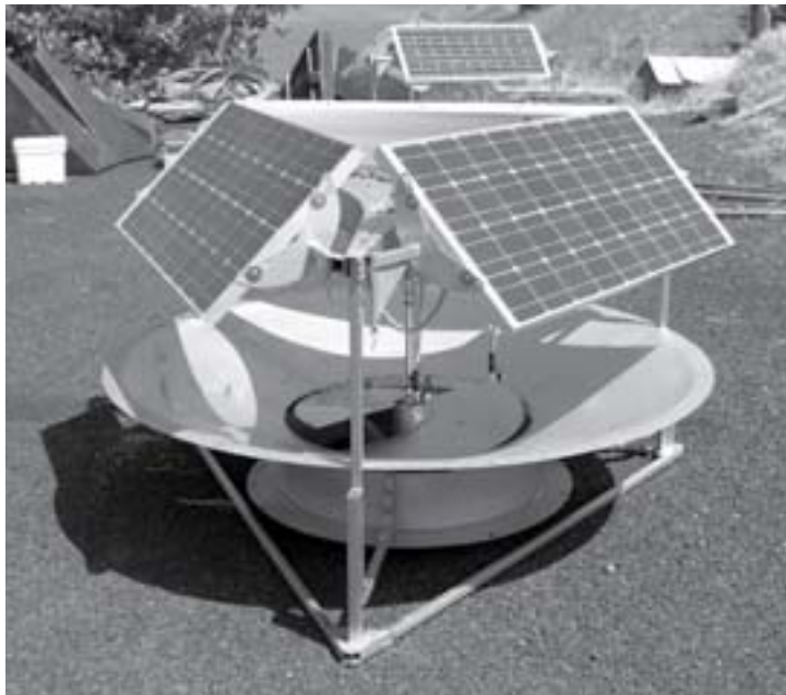
The solar-powered long distance circulator draws water from a specified depth and distributes it throughout the reservoir disrupting blue-green algal habitat.
