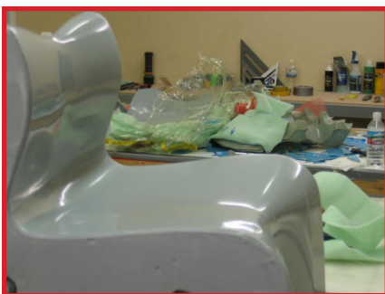
TEPIC tool with gel coat 2 part bolted mold
