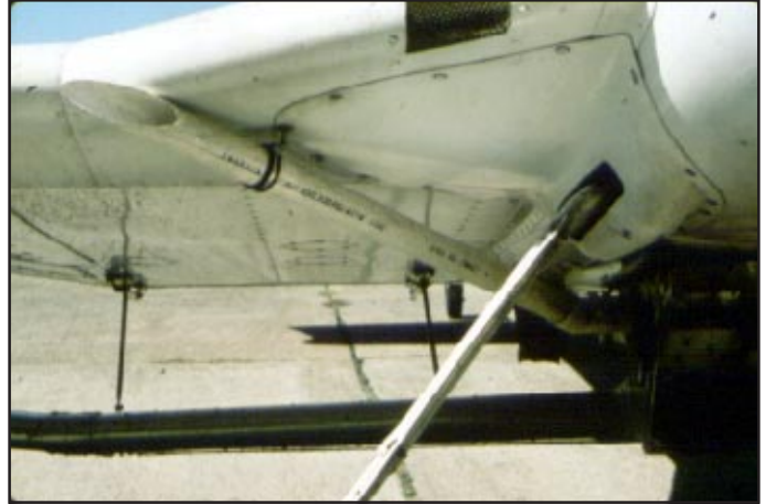
Figures II.18-3 and -4 —Ram air tube fastened to underside of aircraft provides forced air during flight to the air agitation tube.
