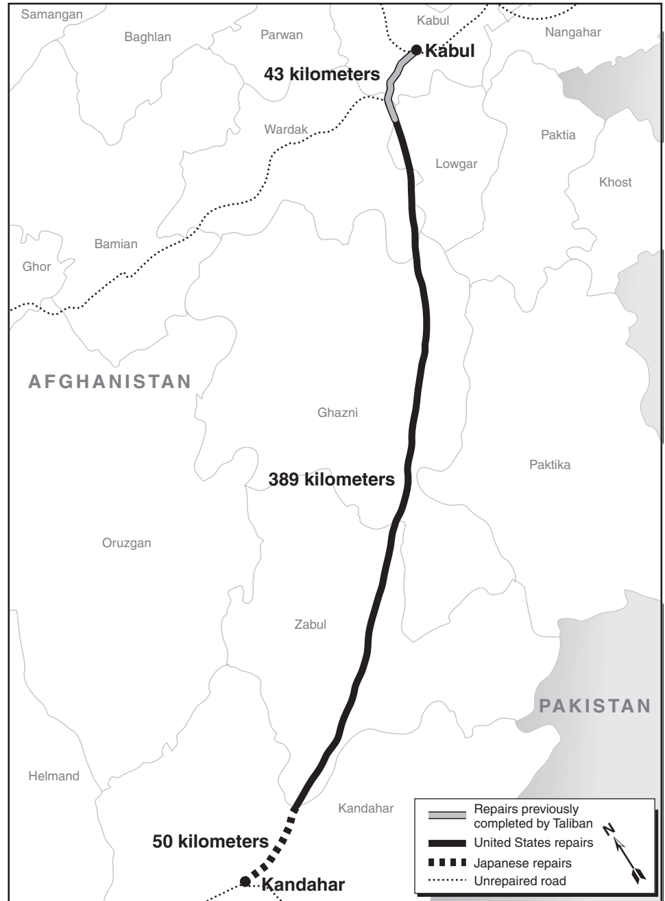
Figure 21: Division of Responsibility for Repairing the 482-kilometer Kabul-Kandahar Highway
