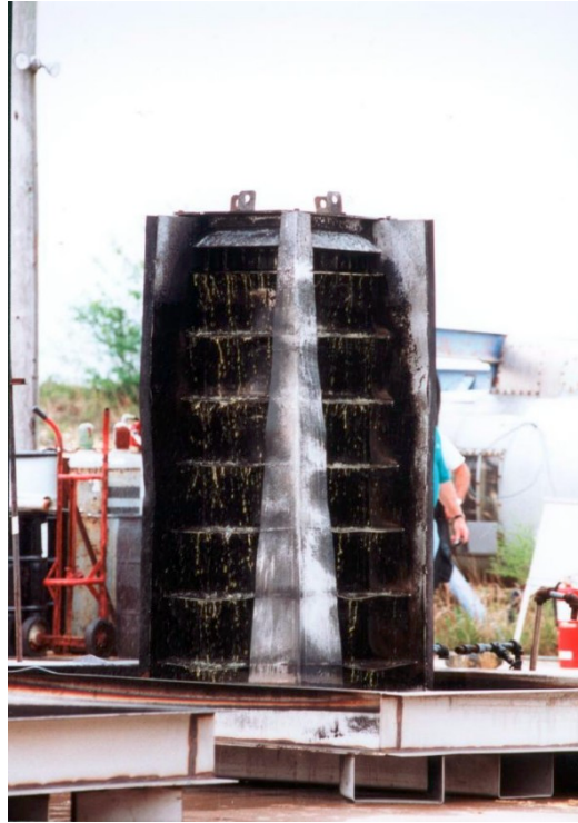
FIGURE 2. THREE-DIMENSIONAL RUNNING-FUEL CASCADE TEST ARTICLE
