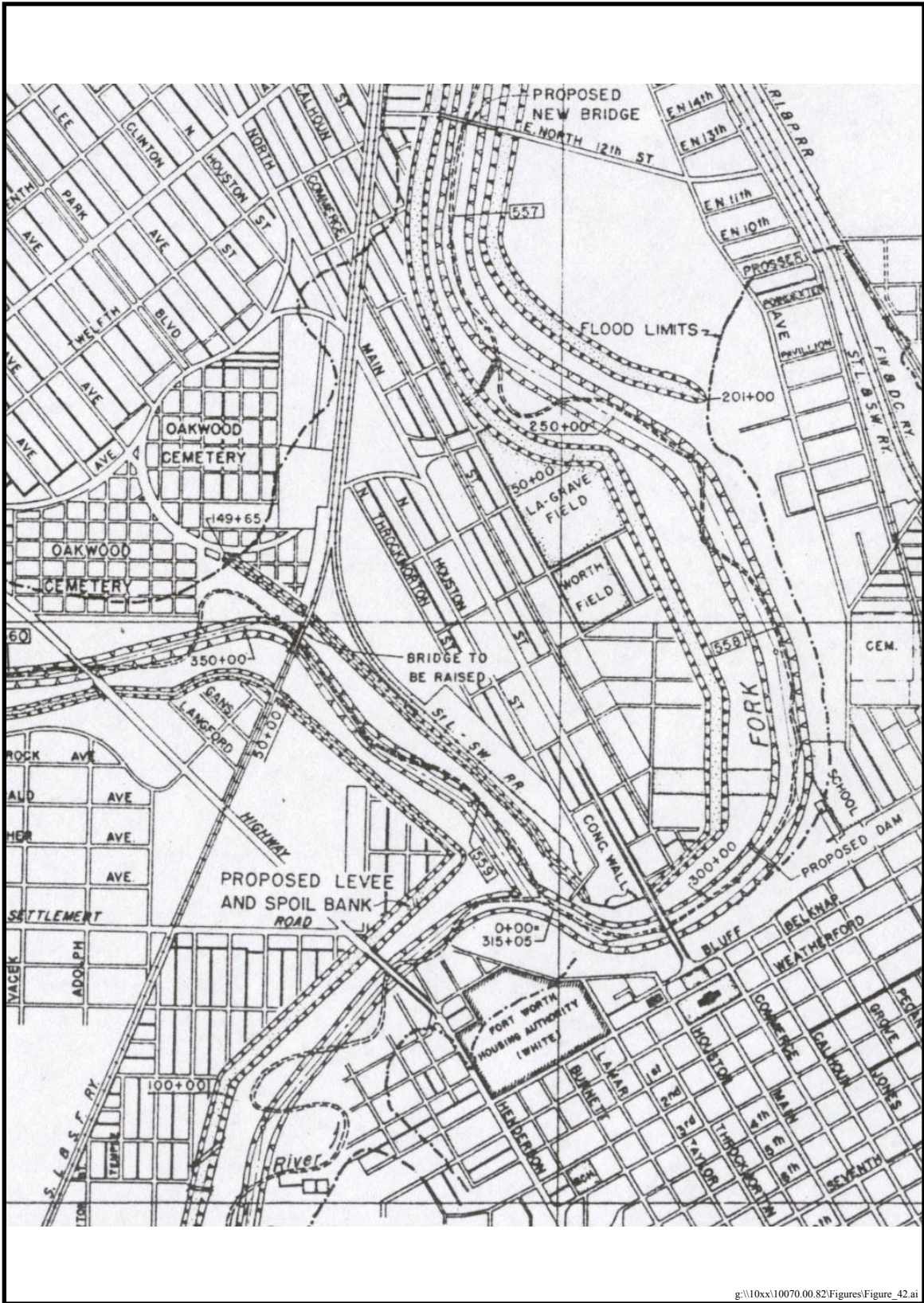
Figure 42. Map with location of proposed levee improvements and channel construction.
