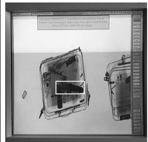
Fictional gun projected into a passenger bag. Note: feedback to the screener is provided in the top box and white highlights.
