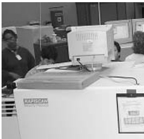
Laboratory acceptance testing of TIP-ready X-ray machines in support of Security Equipment Integrated Product Team procurement.
