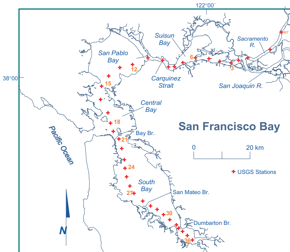
Figure 1. Monitoring of basic water quality parameters. The USGS, in cooperation with RMP, measures basic water quality indicators every month at 38 stations between the Sacramento River and South Bay with additional weekly sampling in the South Bay during spring. Submersible instruments measure salinity, temperature, suspended solids, light penetration, dissolved oxygen, and chlorophyll a from the water surface to the bottom. This basic information provides a foundation for understanding variability in the sources, transport, bioaccumulation, and ecosystem effects of contaminants in San Francisco Bay.
