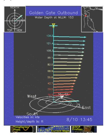
Figure 4. 3-D perspective view of the velocity profile observed by an ADCP deployed in the middle of the outbound lane near Golden Gate showing near surface velocity exceeding 3 knots flowing to approximately  $60^{\circ}$  north.
