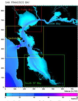
Figure 4. Index map of the San Francisco Bay nowcast numerical model domain. The color background is an index of the water depth.
