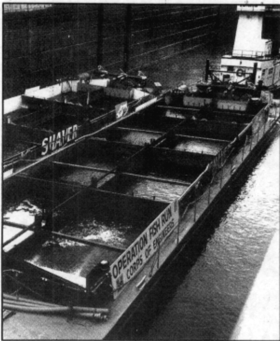
The Walla Walla District began expanding the experimental Operation Fish Run in 1977, instituting a policy of transporting fish by barge.
