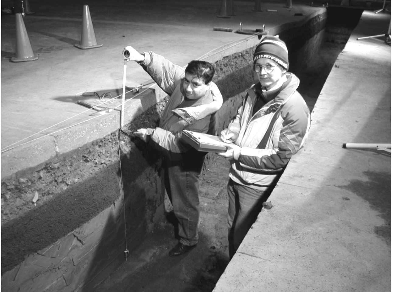
FIGURE 3. PAVEMENT LAYER PROFILE MEASUREMENTS
