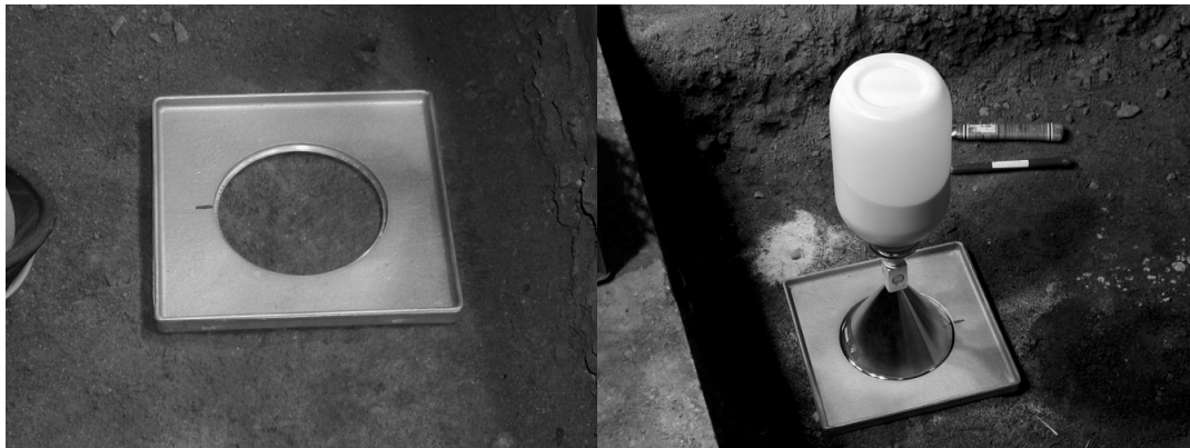
FIGURE 15. SIX-inch SAND CONE TESTS IN P-154 TEST PITS
