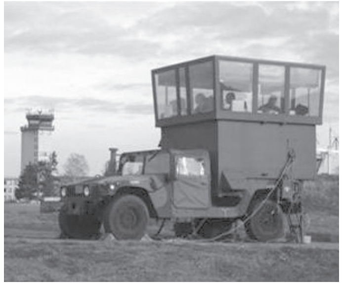
Mobile control tower; a backup capability for continuity of air operations.
