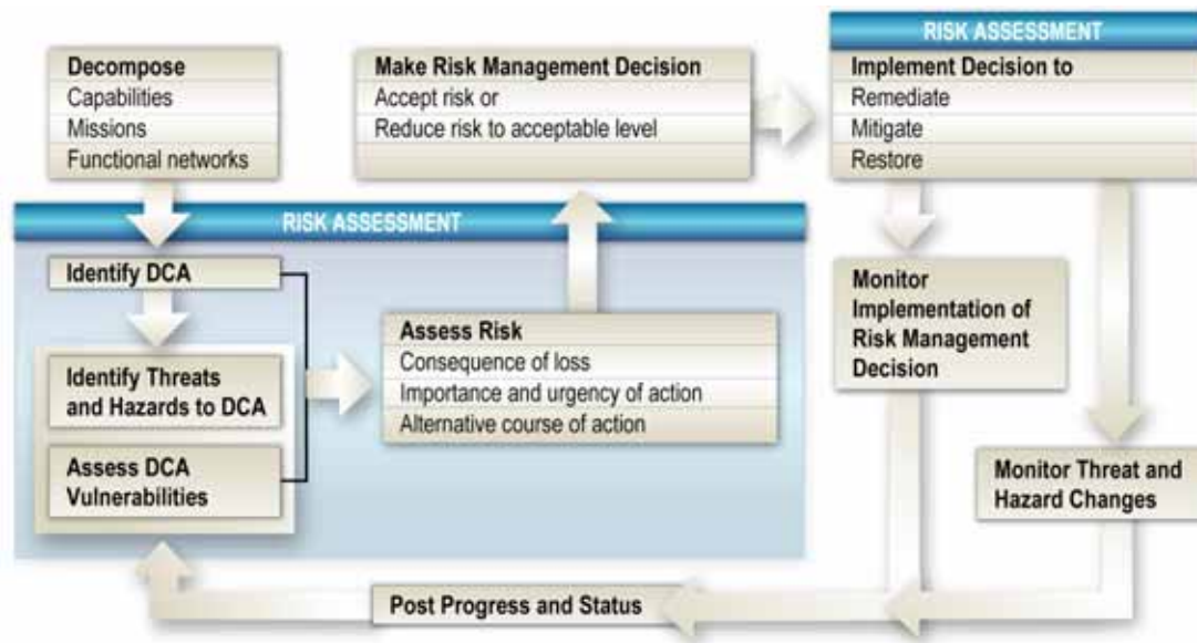
Figure 4.4. DOD Mission-Assurance Process for Critical Infrastructure Protection
