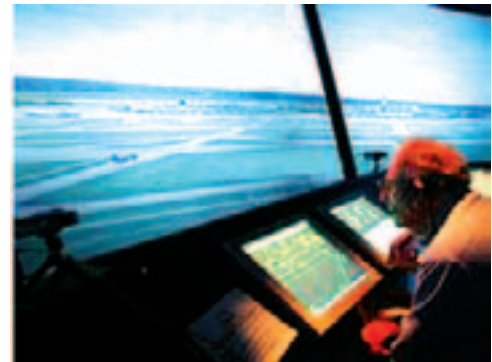
SURFACE MANAGEMENT SYSTEM DISPLAY
