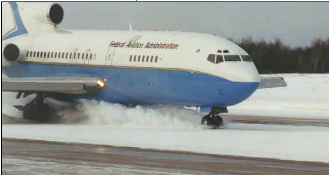
Runway friction test, using the FAA Boeing 727.
