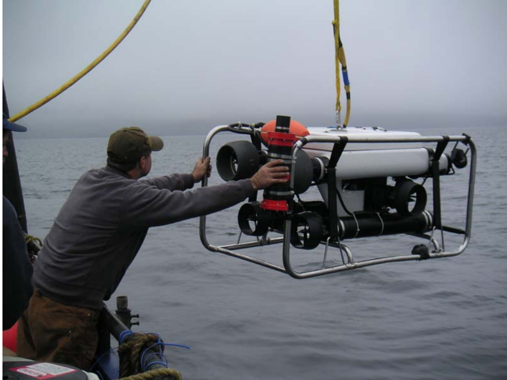
Deployment of remote operating vehicle (ROV).
