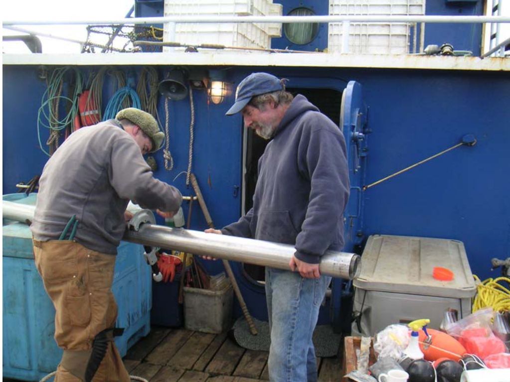
Preparing vibrocore sampling barrel.
