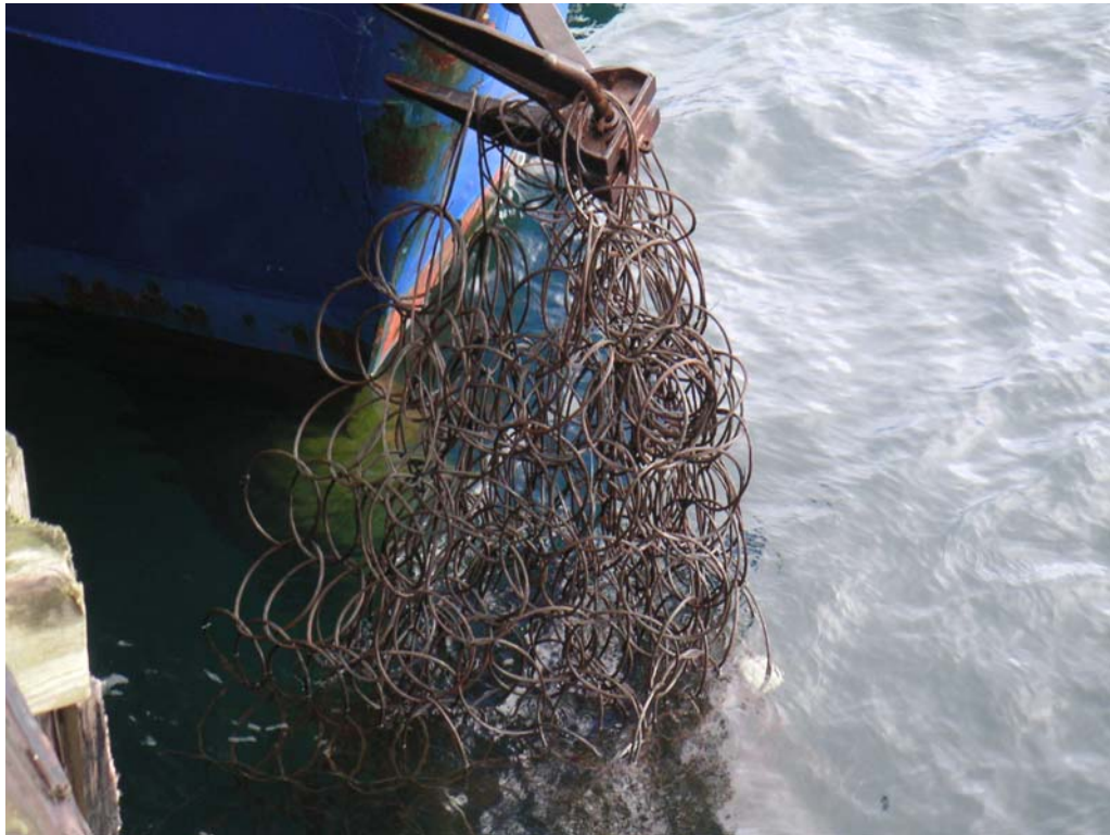
Ship's anchor entangled with WWII submarine net.
