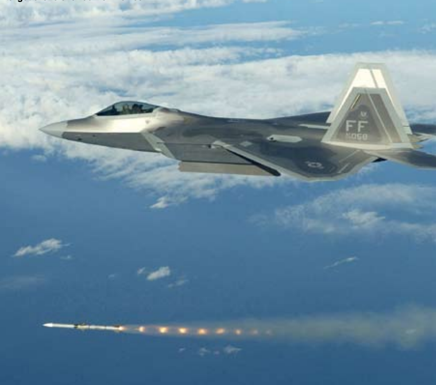
F-22A Raptor fires AIM-120 advanced medium-range air-to-air missile at aerial target drone over Gulf of Mexico
