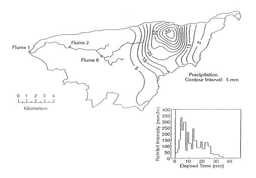
FIGURE 3. Isohyetal map of a storm on August 27, 1982.
