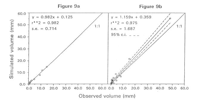
FIGURE 9. Simulated versus observed runoff volumes for Lucky Hills - 106 pretreatment period (1973-1980); a) optimization event set b) verification event set.
