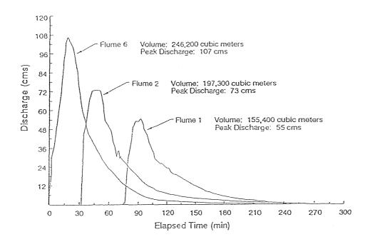
FIGURE 5. Hydrograph resulting from the storm event on August 27, 1982. Transmission losses in the normally dry streambed reduced the volume and peak discharge.
