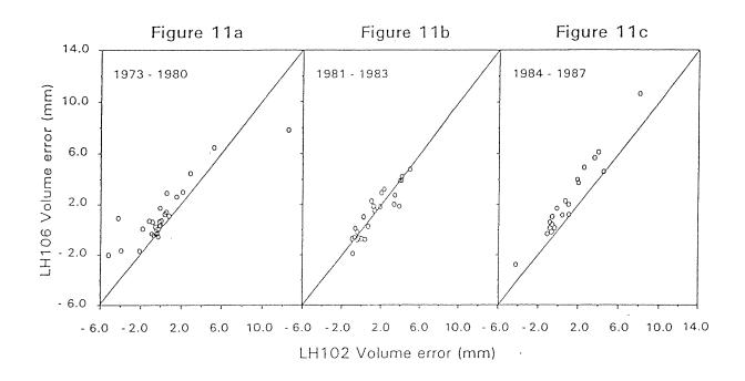
FIGURE 11. Runoff volume simulation errors on LH-106 versus LH-102 for the a) pretreatment period (1973-1980) b) herbicide treatment period (1981-1983) and c) imprint/grass Est. period (1984-1987).
