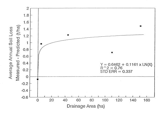
FIGURE 8. Measured minus the RUSLE Average Annual Soil Loss predicted versus watershed drainage area.
