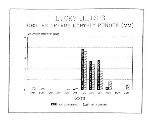
FIGURE 7. Observed and CREAMS simulated runoff for watershed LH-3 (LH-103).
