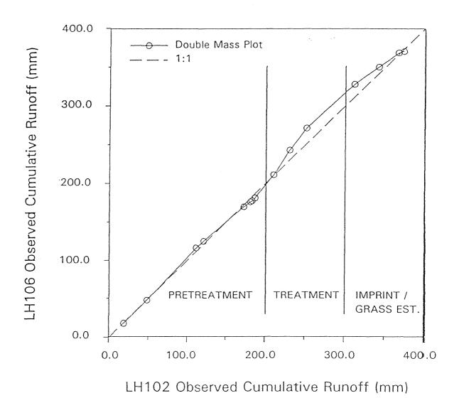
FIGURE 10. Observed double mass plot of accumulated annual runoff volume from LH-102 (untreated) and LH-106 (treated).
