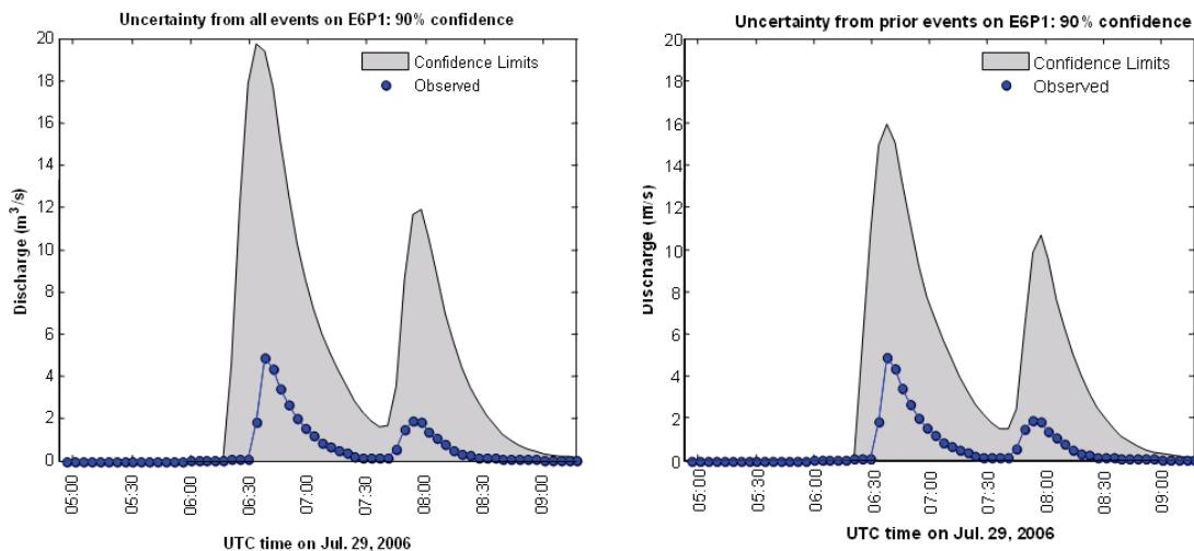
**Fig. 4** Predicted 90% confidence intervals for hydrograph of the 29 July 2006 event using behavioural factor sets from: (a) all events, and (b) prior events. In E6P1, E denotes event and P denotes peak in this multi-peak event.
