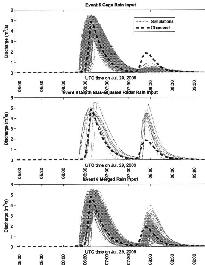
**Fig. 1** Simulations behavioural to the 1st (left) peak examined for their behaviour on the 2nd (right) peak during Event 6 using different rainfall input. Merged case shows more modifier set consistency across peaks, where such consistency is defined as behavioural simulation by the same modifier set across peaks.
