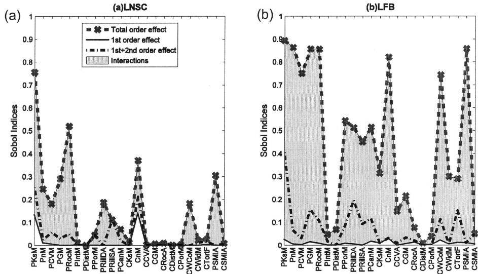
**Fig. 3** Relative influence of model parameters and initial conditions on model response. Subplots show fractional influence on: (a) Nash-Sutcliffe efficiency, and (b) behavioural classification.
