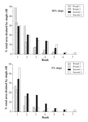
Fig. 4. Area drained by a single rill per treatment and slope determined from the DEM after the fifth rainfall simulation.
