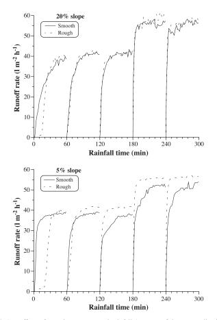
Fig. 2. Runoff rate for each treatment and rainfall (average of the two replications).
