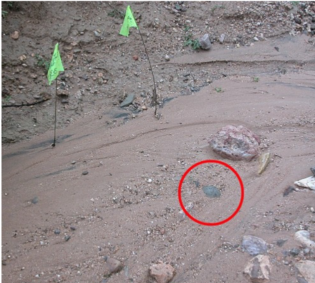
Figure 6. Two buried particles indicated with flags and one exposed particle in the foreground.
