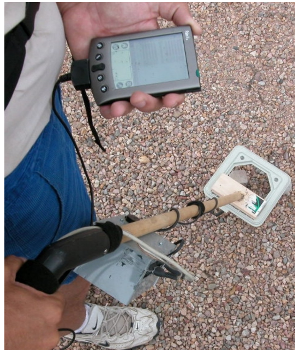
Figure 1. RFID sweeper and portable computer.
