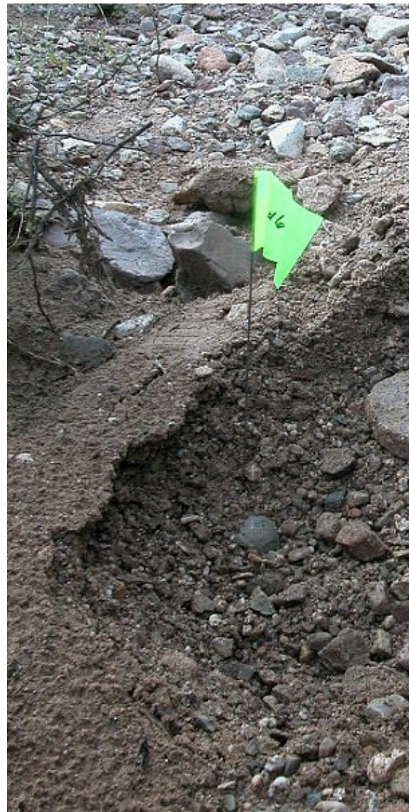
Figure 5. Buried particle exposed for demonstration after detection with RFID system.
