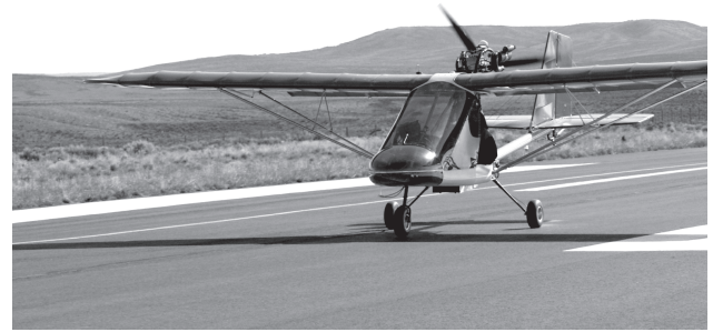
Figure 10. Ultralight airplane used for very-large-scale aerial photography. The sensors are high-shutter-speed film and digital cameras, which are automatically triggered by a computer with an interfaced GPS receiver.
