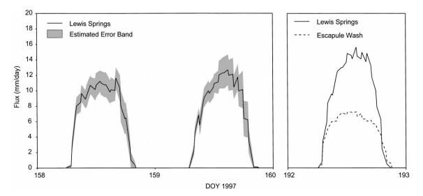
Fig. 5. (Left) scaled sap flow estimates over the 600 m Lewis Springs reach of C/W transpiration for DOY 158 and 159 with estimated error bands; (right) comparison of scaled Lewis Springs versus the ephemeral channel Escapule Wash reach for DOY 192.
