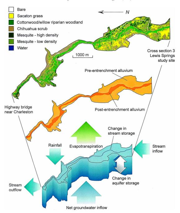
Fig. 3. Riparian corridor for the stream reach from Lewis Springs cross-section 3 to the Charleston, USGS stream gage. (Top) cover classes; (middle) pre- and post-river entrenchment alluvium boundaries; (bottom) primary water balance components for the reach.
