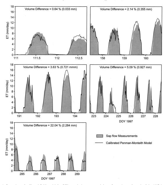
Fig. 6. Comparison of calibrated P-M model for C/W transpiration versus scaled sap flow estimates for each of the 1997 intensive measurement periods.
