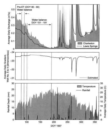
Fig. 4. (Top) streamflow at Lewis Springs cross-section 3 and Charleston USGS gage; (middle) average daily gradient, BLM Well No. 5 to 4 at Lewis Springs; (bottom) rainfall depth and average daily temperature recorded at the Lewis Springs mesquite tower.
