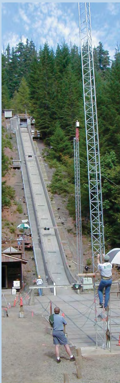
Figure 4. The U.S. Geological Survey (USGS) debris-flow flume is located in H.J. Andrews Experimental Forest, Oregon. The flume was constructed to conduct controlled debris-flow experiments. Photograph courtesy of the USGS, taken September 13, 2001.
