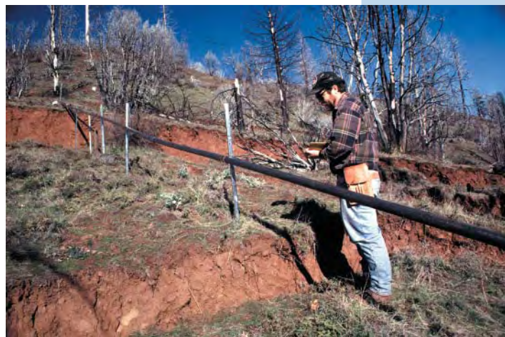
Figure 7. Measuring landslide movement. Photograph by Richard LaHusen, U.S. Geological Survey.
