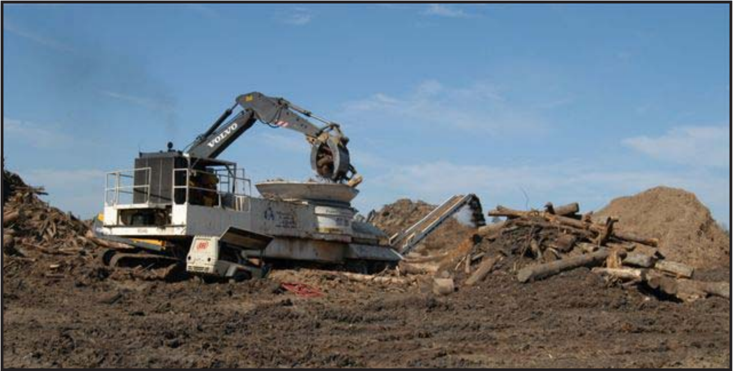
Debris being “chipped” at the Orange County reduction site.
