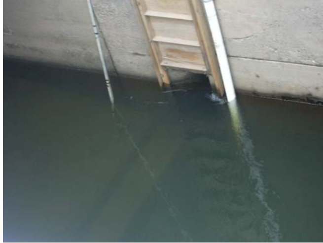
Figure 1. Overhead view of the Mill Creek Diversion Dam fish ladder exit. The underwater camera was attached to the pipe on the left side of the photo and a water quality monitor was located in the white pipe on the right side of the photo.
