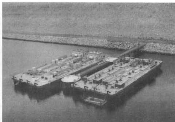
Figure 1-7. Fish barges (two 86,000 gal, two 100,000 gal, and two 150,000 gal capacity) used in the juvenile fish transportation program.
