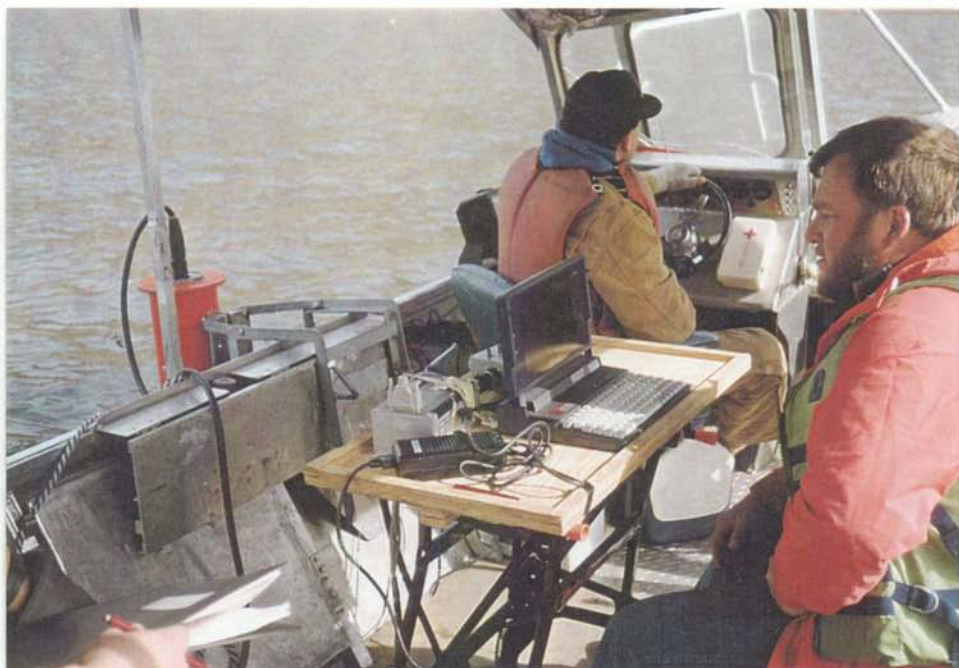
Figure 8. Close-up of USGS crew operating a computer which records transmissions from the Acoustic Doppler Profiler (red cylinder mounted on side of boat).
