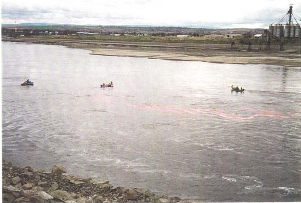
Figure 1. Releasing Dye at River-Mile 138.34.
