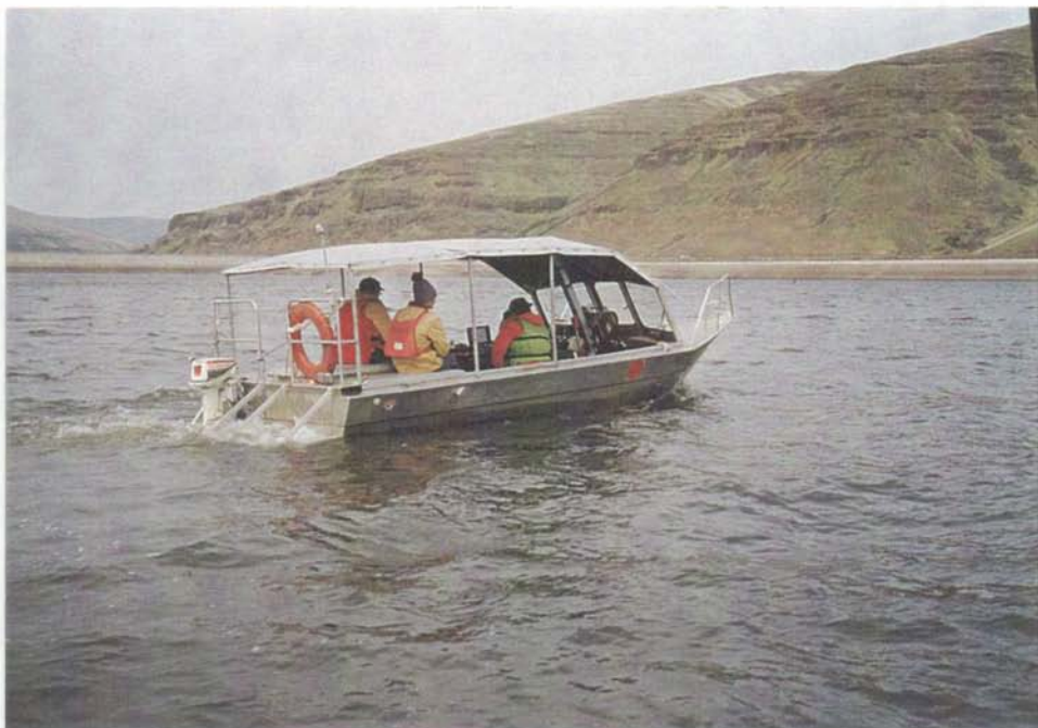
Figure 7. USGS boat recording water velocities as it moves across the river along a sediment range line.
