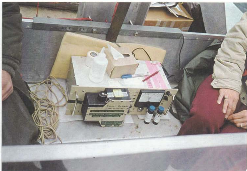
Figure 4. Fluorometer instrument used to measure dye fluorescence.
