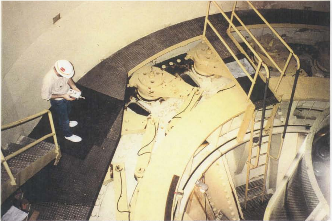
Photo No 10 - Noise level readings in turbine pit using hand held meter. - Lower Granite Dam and Powerplant, Pool Lowering Test, March 1992.
