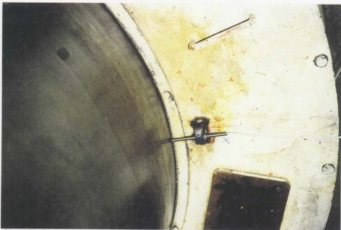
Photo No 6 Winter-Kennedy measure using differential pressure transducer. - Lower Granite Dam and Powerplant, Pool Lowering Test, March 1992.
