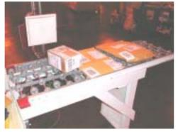
Small packages are individually run in front of a reader on a gravity conveyor.
