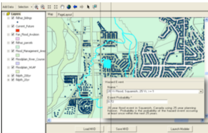
Using the Land Use Portfolio Model to assess the risk of flooding in Squamish, British Columbia. Black dots show buildings at risk of flooding in a simulated 20-year flood.
