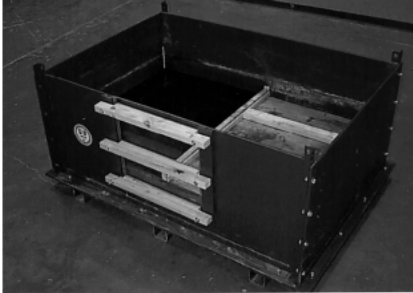
FIGURE 7-6. PHOTOGRAPH OF COMPLETED REACTION BOX
