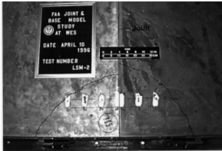
FIGURE 7-30. POSTTEST PHOTOGRAPH OF SLAB TO SURFACE, EXPERIMENT LSM-2
