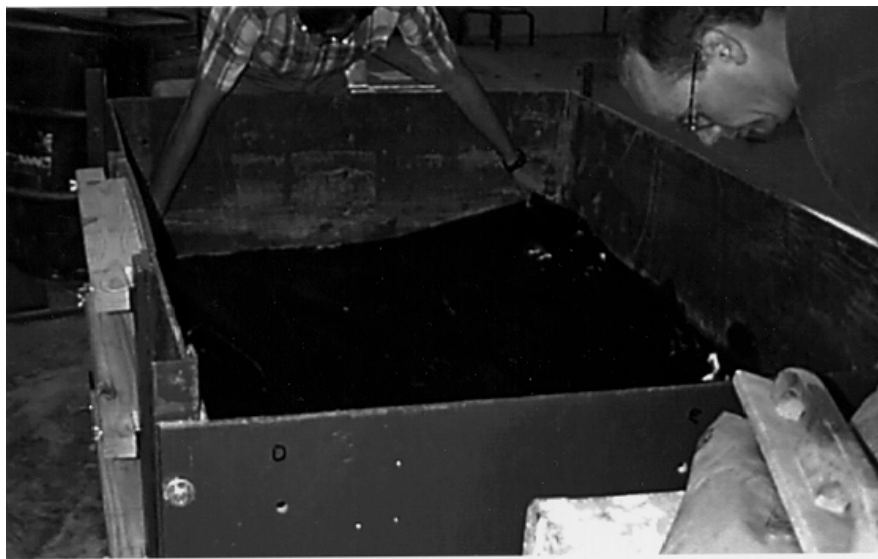
FIGURE 7-8. INSTALLATION OF POLYETHYLENE FILM IN REACTION BOX
