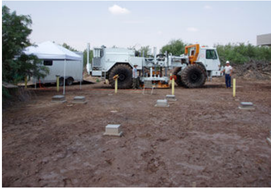
The University of Texas NEES T-REX tri-axial shaker inducing liquefaction in the saturated soil deposit at the NEES Wildlife Liquefaction Array, in Imperial Valley, CA. The liquefaction array is operated by the University of California, Santa Barbara. Image courtesy of the University of Texas.
