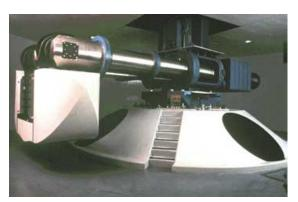
with instrumented physical models. Commissioned in 1995, the centrifuge supports research investigations in the fields of geotechnical, structural, coastal, hydraulic, and environmental engineering, in addition to blast and infrastructure protection. Studies are possible under a wide range of climatic conditions.
