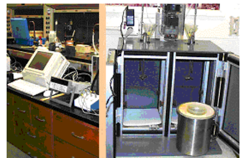
Calorimetry instrumentation for analyzing cement reaction rates and effects of admixtures
