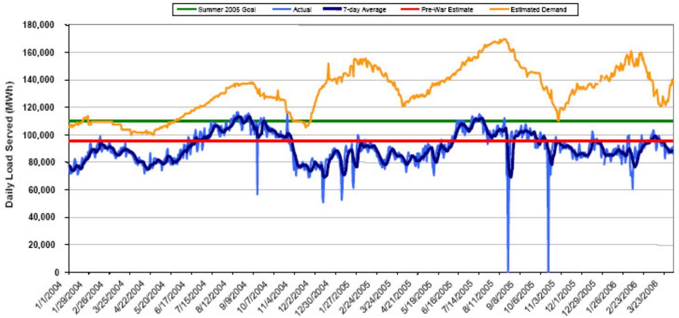
Figure 5: Estimated Daily Electricity Produced in Iraq, January 1, 2004-March 23, 2006
