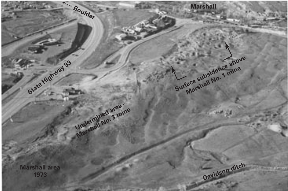
Figure 23. Oblique aerial photograph (looking northwest) showing surface subsidence features caused by the collapse of underground coal mines near the town of Marshall, Colorado, in 1973. Photograph courtesy of R.B. Colton (scientist emeritus), U.S. Geological Survey, Denver, Colorado.
